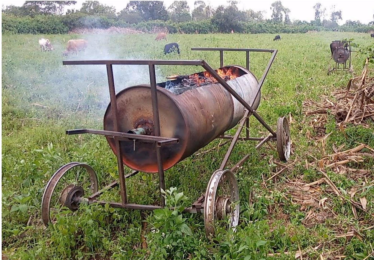
These are H-Frame kilns, the preferred design for fabrication. The "H" is seen at both ends of the kiln.
